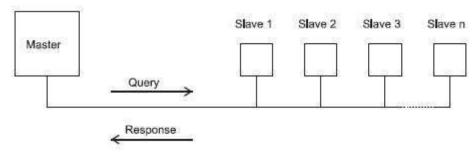
In the MODBUS Protocol the master can address individual slaves, or, using a special "Broadcast" address, can initiate a broadcast message to all slaves. The Eastron Digital meter do not support the broadcast address.
