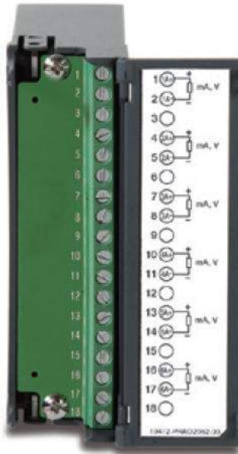
**Note 1:** The IO Cards should not be removed or Inserted to the PR when the Power is ON. This should be carried out in the Power OFF Condition only.
