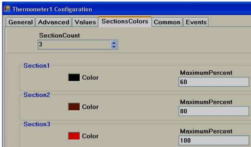
**Section Colors:** Define bands to display Ticks and Label color accordingly based on the value of the tag during Run time.
