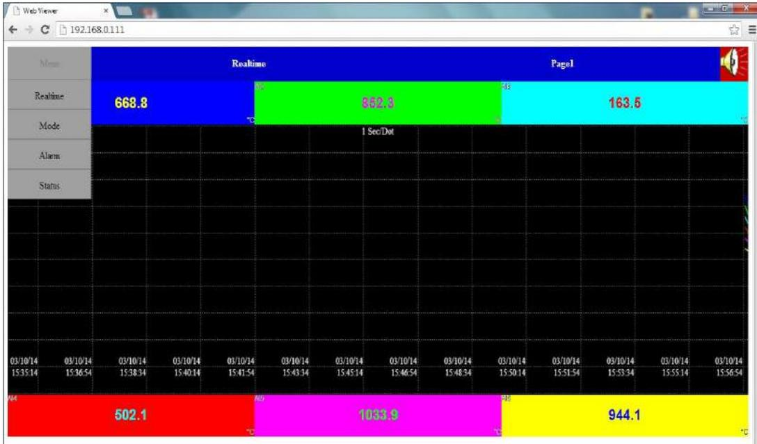
The display includes Real time values of all channels like AI, Math, Counters, Totalizers, Real time alarms, historical alarms, status of Digital Inputs, Digital Outputs, Analog Outputs, Counters, and Totalizers etc...
