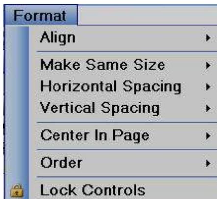
**Align:** Used to align selected components, objects etc. for adjusting their position precisely in the screen layout. Available options for selection are Center, Right, Left, Top, middle & Bottom.
