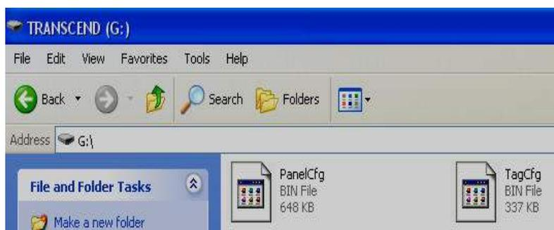
3. Remove the removable media from the recorder. Insert into PC
