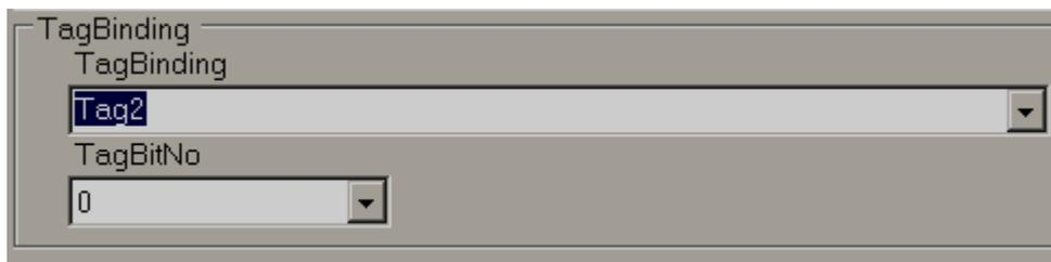
In the above figure, Tag2 is an analog type (4 byte), so, a TagBitNo combo box will appear for the selection of the required bit within 32 bits (0 to 31).
