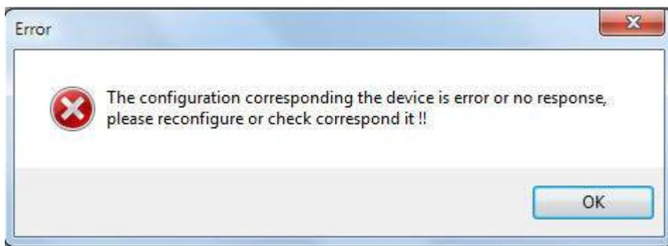
If this is the case, please check the Ethernet cable connections at both the Recorder and PC/LAN HUB side. Also make sure that green communication LED is lit which shows there is a proper firm connection at the RJ 45 connector.
